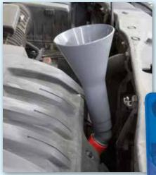
When combined with our other adapters, the 45° elbow extension allows where funnels otherwise do not fit
